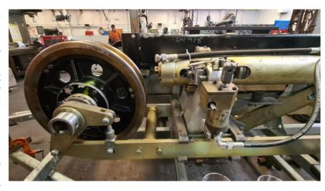
understanding of the condition and remaining service life of all the bogies. During this process, all safety systems are tested to the appropriate standards to ensure that they continue to meet their original performance requirements.
